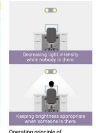
Operating principle of human-detecting sensor
