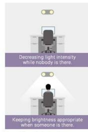
Operating principle of human-detecting sensor
